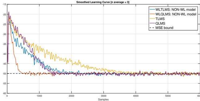
**Fig. 3.** MSE: (WL-)QLMS vs (WL-)TLMS with Ambisonic improper input signal. *NON-WL model* in the legend box refers to a system to be identified which only has  $\mathbf{w}_0$  weights.
