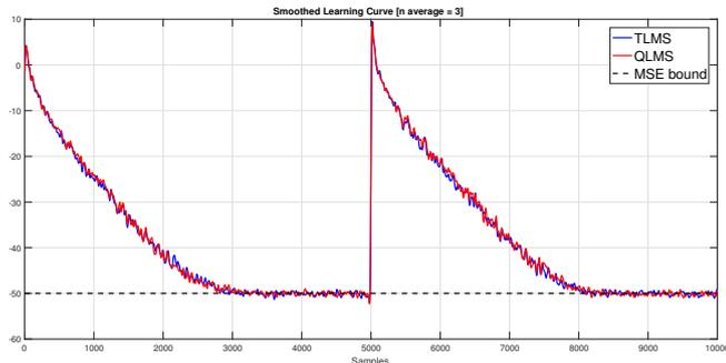
Fig. 2. MSE: QLMS vs TLMS with proper input signal.
