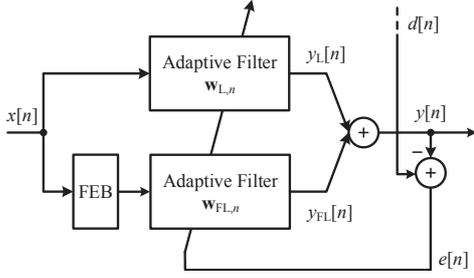
**Fig. 1.** The split functional link adaptive filter.
