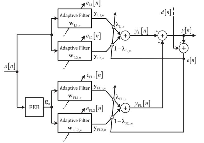
**Fig. 3.** The proposed filtering scheme where the filter block outputs are combined by the mixing parameter vectors.
