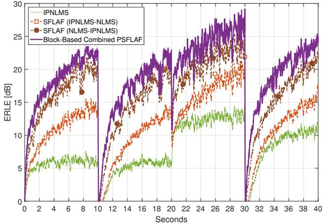
**Fig. 4.** Performance behavior in terms of the ERLE in case of colored noise as input.
