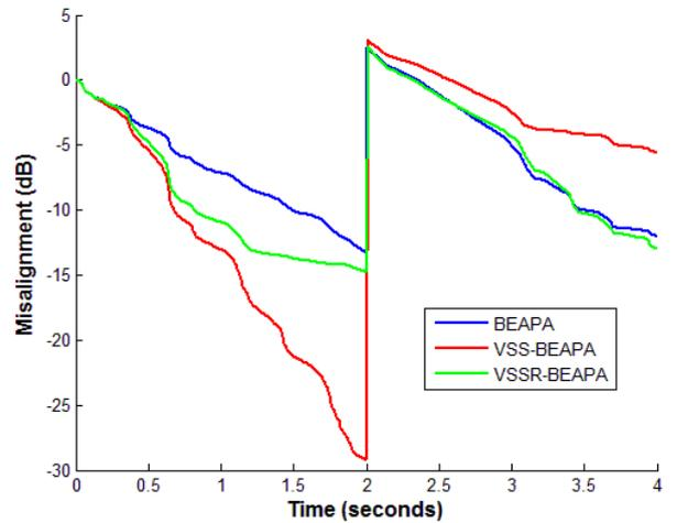
Figure 3. Misalignment of BEAPA, VSS-BEAPA, VSSR-BEAPA. The input signal is a speech sequence,  $P = 2$ ,  $L = 512$ , and variable background noise (SNR decreases from 25 dB to 15 dB between times 1s and 2s, otherwise is 25 dB).
