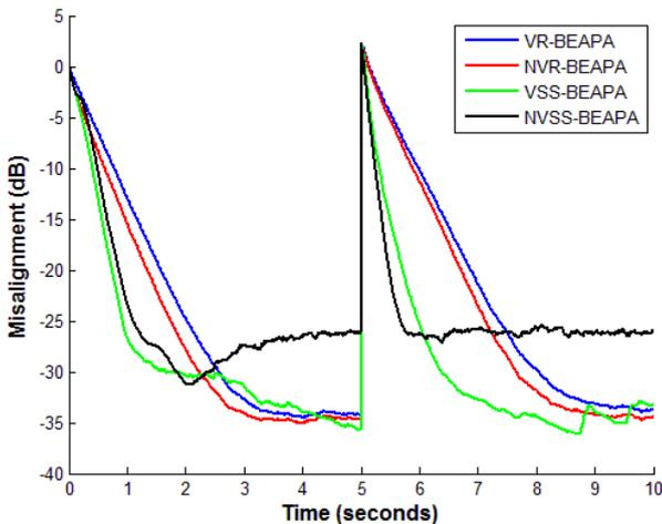
Figure 1. Misalignment of VR-BEAPA, NVR-BEAPA, VSS-BEAPA, NVSS-BEAPA. The input signal is a colored noise sequence,  $P = 2$ ,  $L = 512$ , echo path changes after 5 seconds, SNR= 30 dB.
