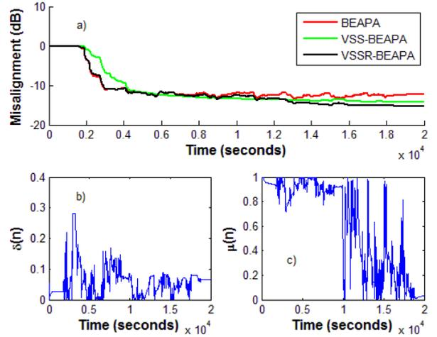
Figure 2. The input signal is a speech sequence,  $P = 4$ ,  $L = 300$ , SNR= 20 dB. a) Misalignment of BEAPA, VSS-BEAPA, VSSR-BEAPA; b) The variable regularization factor of VSSR-BEAPA; c) The variable step size of VSSR-BEAPA.
