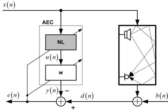
**Fig. 2.** The proposed Hammerstein NAEC architecture.
