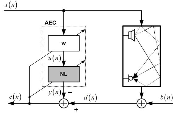
**Fig. 3.** The proposed Wiener NAEC architecture.
