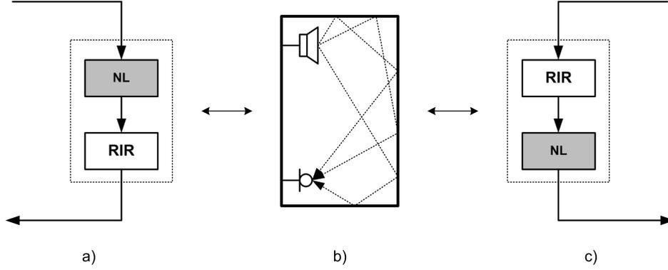
**Fig. 1.** Two different implementations of a distorting echo path (b): (a) cascade of a nonlinear function (NL) and a Room Impulse Response (RIR) (Hammerstein system) and (c) cascade of a RIR and a NL (Wiener system).
