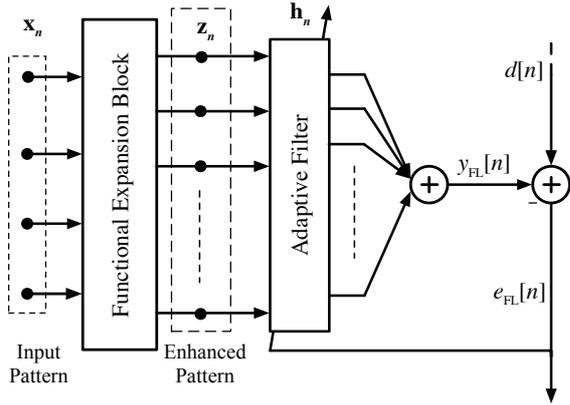
Fig. 1. The Functional Link nonlinear filter.
