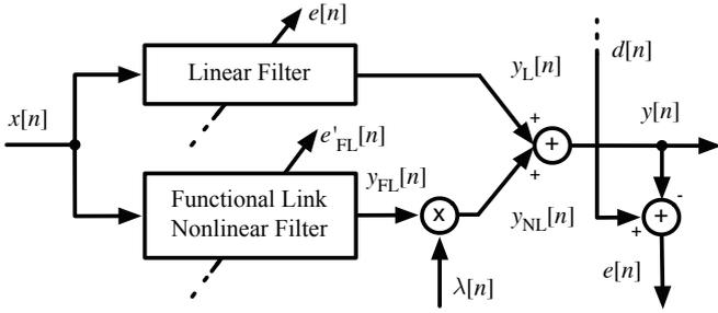
**Fig. 3.** “NLMS-FL/AZK” architecture: linear combination between an NLMS linear filter and a nonlinear filter composed of a convex combination between an FL nonlinear filter and an all-zero kernel.
