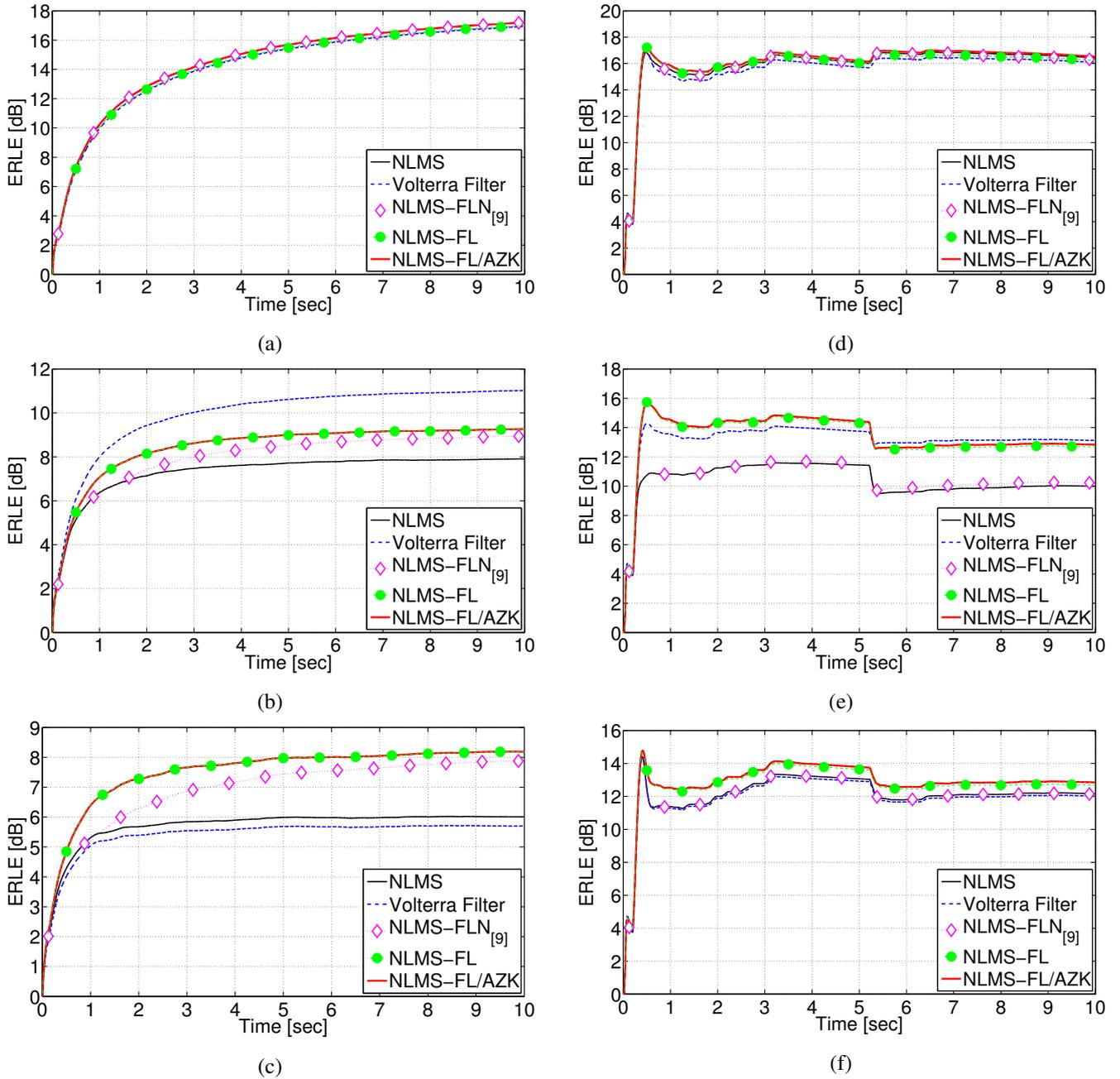
**Fig. 4.** Performance of the described architectures in three different scenarios: (a),(d) linear path, (b),(e) linear path with quadratic distortions, (c),(f) linear path with soft clipping. Two different signals are used as input: (a),(b),(c) white Gaussian noise and (d),(e),(f) female speech.
