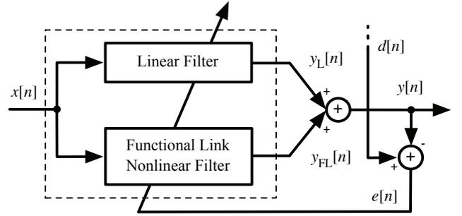
Fig. 2. "NLMS-FL" architecture: linear combination between a NLMS linear filter and a FL nonlinear filter.
